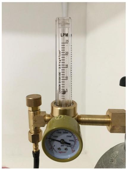
The image above shows the flow meter in action - this particular meter is set to ~5 liters per minute, as indicated by the ball bearing hovering at that mark. The pressure gauge with the
